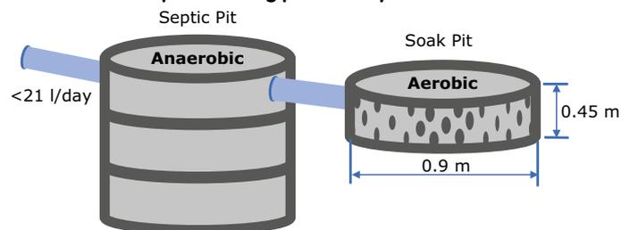
Figure 6: Installation of a second offset pit in very fine sandy soil in the terai where pits are filling prematurely
