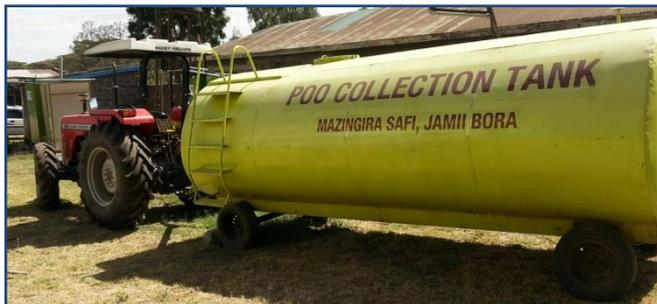
Photo 6: The mobile sludge transfer station
