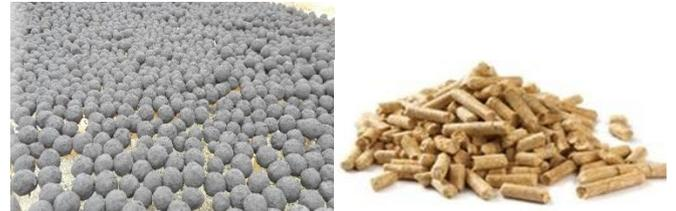
Photo 9: Carbonised briquettes (left) and non-carbonised pellets (right)
