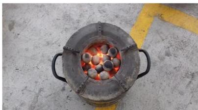
and biomass-fuels-briquettes made partly from human waste and sawdust. Carbonised round shaped briquettes were chosen and currently the production is being up-scaled.
