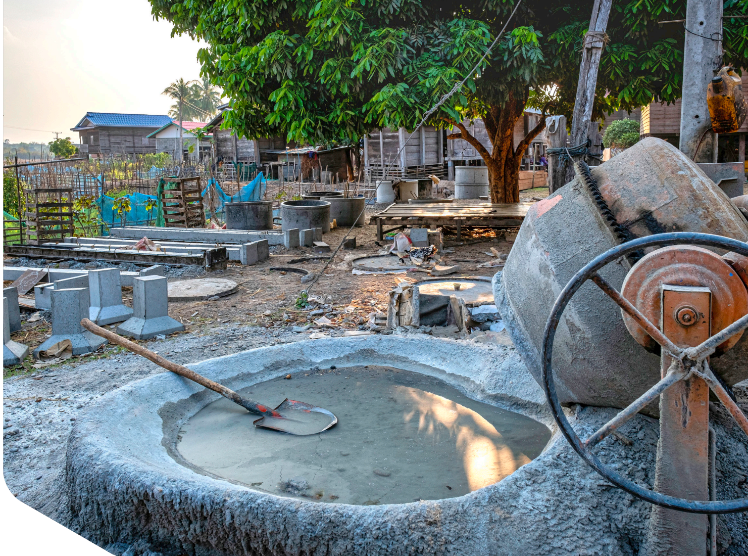
Photo: A sanitation enterprise producing concrete rings to store latrine waste.
